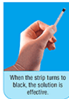
With no change of colour to the strip, solution needs to be changed.
